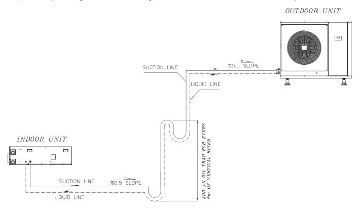
• If the indoor unit lies above the outdoor unit, the suction line must have a loop at the indoor unit's outlet to prevent refrigerant from draining into the compressor during off-cycles.
